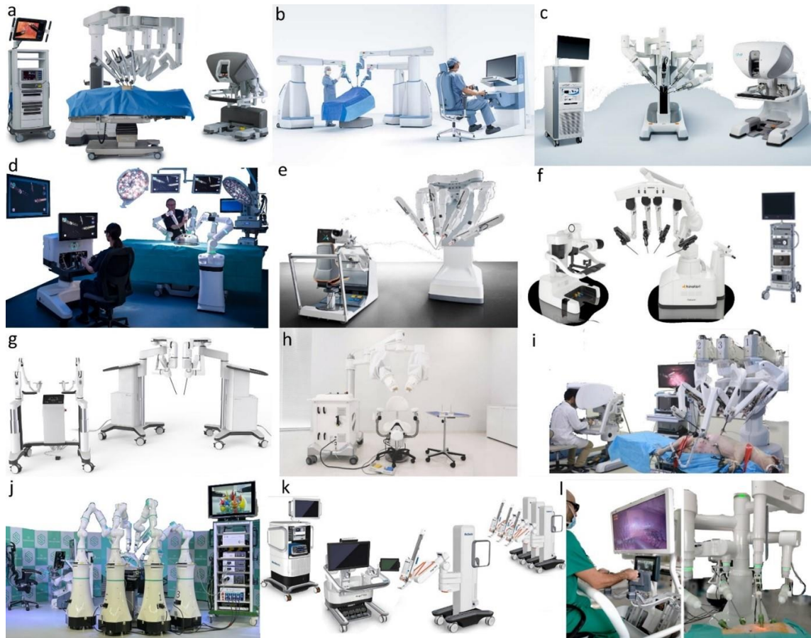
2.2. Figure: The most advanced RAMIS systems, featuring only commercially available, and ready-to-launch platforms, already cleared for at least a limited set of surgical indications (presented in the order of time of appearance). A) da Vinci Xi, b) Senhance Surgical Robotic System c) Revo-i, d) Versius, e) avatera, f) hinotori, g) Dexter, h) Symani Surgical System, i) Toumai Endoscopic Robot, j) Mantra, k) Hugo RAS System, l) Bitrack. Table I provides details regarding these robots' basic engineering and clinical capabilities [17].
