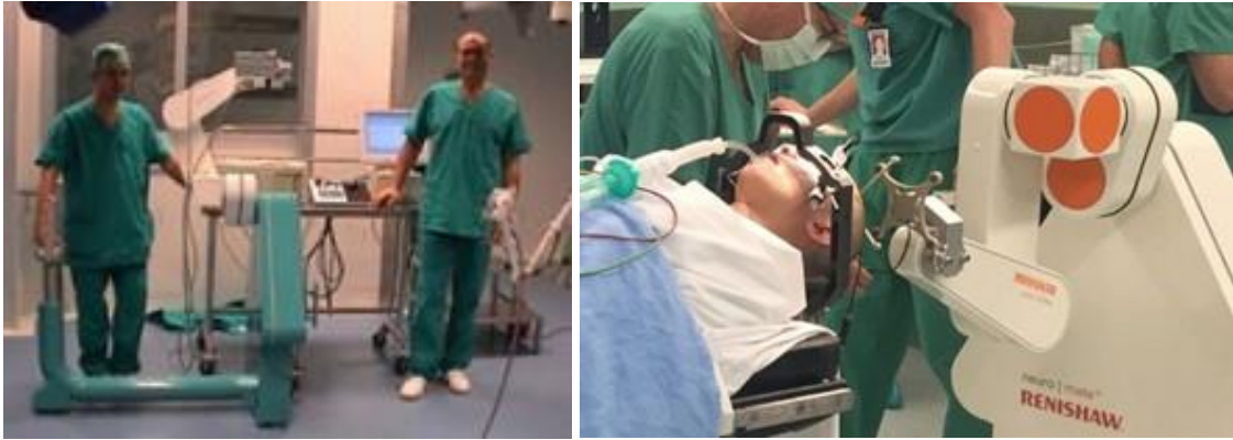
2.4. Figure: a) The first clinically used (1998) and b) the current, commercially available version of the neuromate robot being set up for stereotactic brain biopsy. (Credit: Renishaw plc.)
