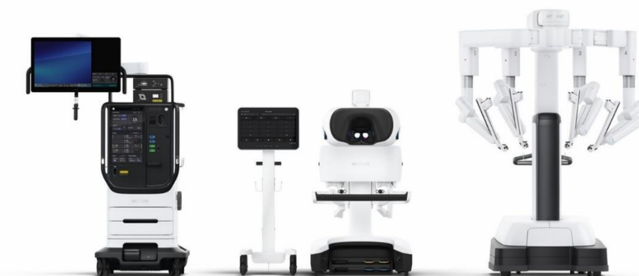
2.1. Figure: The flagship of the RAMIS systems, the newest generation da Vinci 5 from Intuitive with the redesigned surgeon cockpit and the patient-side manipulators. (Image credit: Intuitive Inc.)
