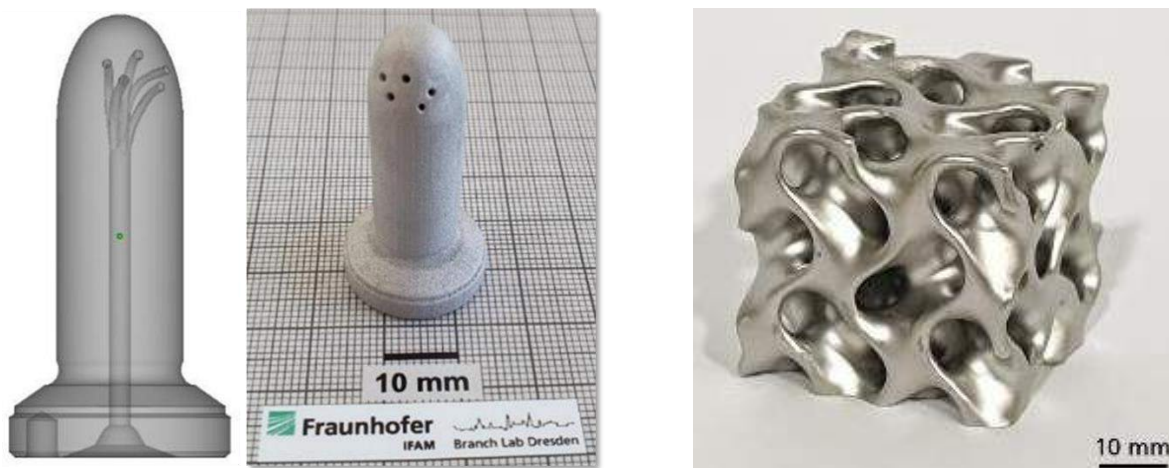
Figure 1. Printed injection nozzle made of 713c using MoldJet (left), excellent surface quality without post processing using 3D Gel Casting (right)
