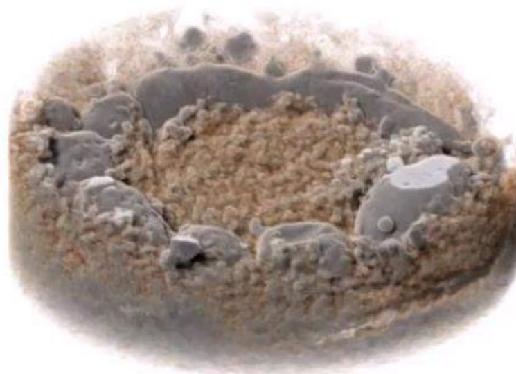
Figure 1. LPBF of AlSi10Mg powders observed with X-ray tomography operando, time-resolved and in 3D during formation.
