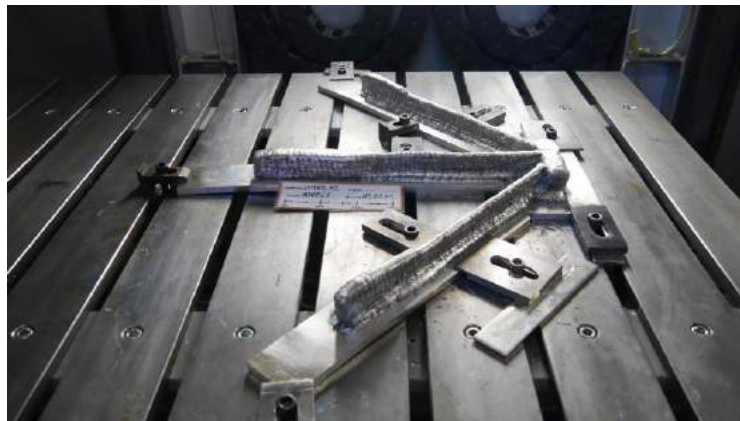
Figure 1. Magnesium alloy AZ91 demonstrator deposited via Plasma Metal Deposition (PMD).
