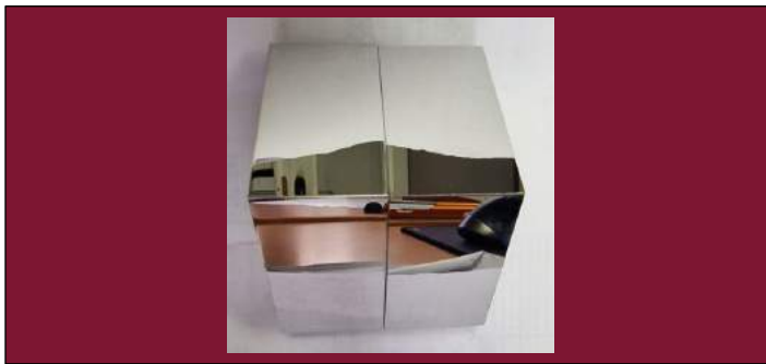
Figure 1. 60mm*30mm*60mm (L*W*H) sample after polishing showing mirror finish, printed in Printdur HCT on FormUp350.
