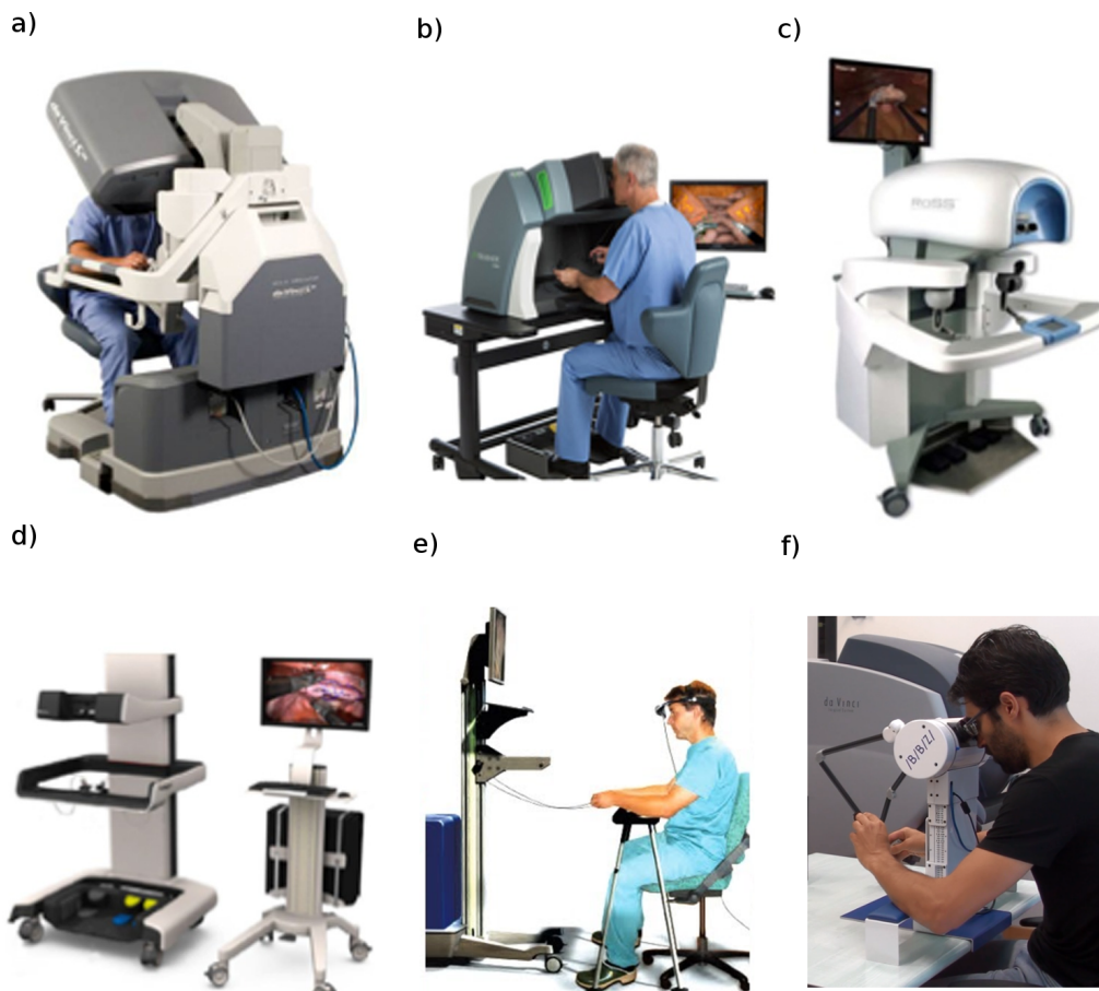
Fig. 3.1. Virtual reality simulators for the da Vinci Surgical System [7, 8, 9]. A) da Vinci Skills Simulator (Intuitive Surgical Inc.), b) dV-Trainer (Mimic Technologies Inc.), c) Robotic Surgery Simulator (Simulated Surgical Sciences LLC), d) Robotix Mentor (3D systems), e) SEP Robot (SimSurgery), f) Actaeon Robotic Surgery Training Console (BBZ Srl).
