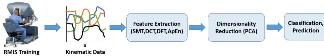
Fig. 3.4. Flow diagram for automated surgical skill assessment proposed by Zia et al. [11].
