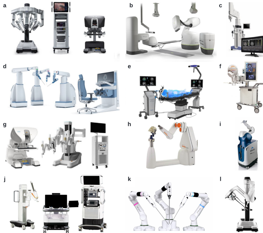
Fig. 1.2. Commercialized, ready-to-launch and research robotic surgical systems along the three main control types (teleoperation, cooperative, image-guided). A) Da Vinci Xi (Intuitive Surgical Inc.), b) CyberKnife (Accuray Inc.), c) TSolution One (THINK Surgical Inc.), d) Senhance Surgical Robotic System (Asensus Surgical), e) iSYS/Micromate/Stealth autoguide robot (Medtronic), f) Eigen ARTEMIS (Eigen Health) g), Revo-i (Meerecompany), h) Neuromate (Renishaw), i) Mako (Stryker Corporation), j) Hugo RAS system (Medtronic), k) Versius (CMR Surgical), l) da Vinci SP (Intuitive Surgical Inc.).
