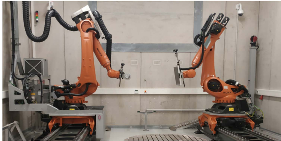
Figure 11. Twin robotic CT system of the Deggendorf Institute of Technology at the Technology Campus Plattling.
