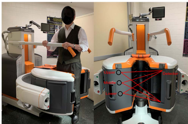
Figure 4. Illustration of the three-source Carestream CBCT scanner installed at Imaging for Surgery, Therapy and Radiology (I-STAR) laboratory, Johns Hopkins University. Upper, Middle and Lower denote the upper, middle, and lower x-ray sources, respectively.
