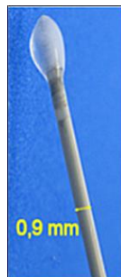
Left: Micro cryo sond with ice ball Right: Assembly of samples in the clean room
